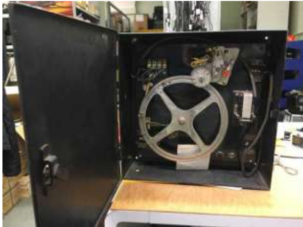
Time synchronisation unit, ca 1938. Built by Watson Norsk AS.
